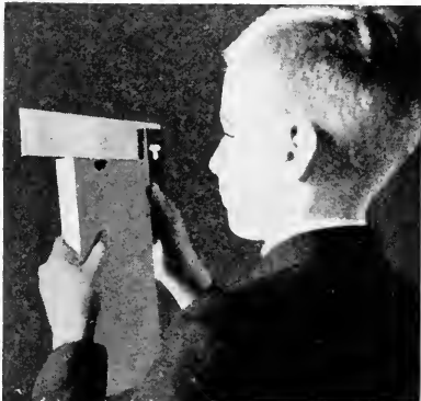
Fig. 6. Testing to See if End is Square with the Edge.
